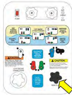
Sewer Tank Flush Inlet on Utility Center
